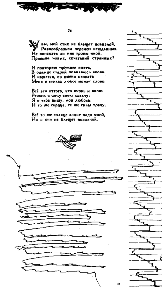
Fig. 125. Record of the eye movements of a subject reading a Shakespeare sonnet. Record on stationary photosensitive paper (a) and on moving phototape of a photokymograph (b).
